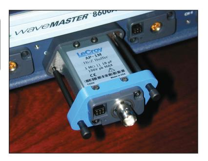
The AP-1M accessory offers a convenient method to provide a high impedance input when using a WaveMaster series instrument, including the DDA5005 and SDA series. Applications which combine one or more high speed signals along with the need to look at larger voltage, slower signals will benefit from the AP-1M which provides a 1 Megohm input impedance path and a full scale range
